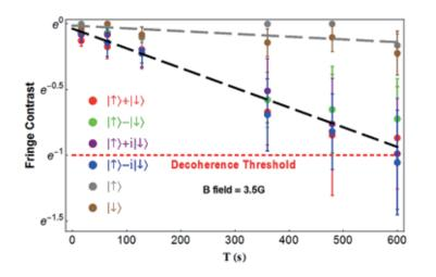
The experimentally measured coherence times of ion with six different initial states
