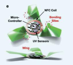
A 3D IoT macroflier with a circuit to measure fine dust pollution through a light dosimetry method.
